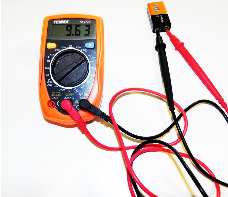
Figure I. A multimeter measuring a battery voltage.
